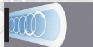
Standard Shroud Airflow is more diffused
