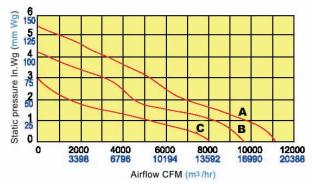
A=80 psig (5, 6 kg/cm²) at large nozzle or 150 psig (10,6 kg/cm²) at small B=60 psig (4, 2 kg/cm²) at large nozzle or 115 psig (8, 1 kg/cm²) at small C=40 psig (2, 8 kg/cm²) at large nozzle or 80 psig (5, 6 kg/cm²) at small
